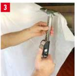
Now press the release button and pull the telescopic rod out until the support surface and the ceiling touch. Then pull the lower part of the foil under the support surface of drywall support on the floor.
