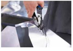
Shape and straight cutting snips D27A
