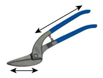
In standard tin snips, edges and handle are traditionally forged into one unit. The force required for cutting is determined by the ratio of edge length to the handle length.
