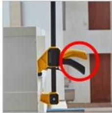
**The risk of damage to the workpiece and injury** increases in cramped working areas when clamping tools with protruding components are used.
