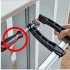
**Clamping in a narrow section** can cause problems when using classic screw clamps and lever clamps as the handle prevents the clamp from being placed correctly.
