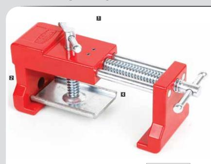
The cabinetry clamp is designed to combine the multiple steps of face frame cabinet installation into one easy process. Face frame stiles can be tightened, aligned, pre-drilled and fastened while the clamp is in place. The clamp holds the individual cabinet edges together while also keeping the faces along the
