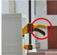
**The risk of damage to the workpiece and injury** increases in confined working areas when clamping tools with protruding components are used.
