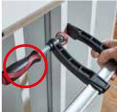
**Clamping in a narrow section** can cause problems when using classic screw clamps and lever clamps as the handle prevents the clamp from being placed correctly.
