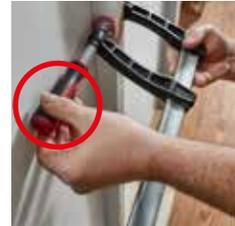
**The clamping in front of a closed surface** is not possible due to the positioning of the handle with classic screw clamps and lever clamps as the handle cannot be actuated.
