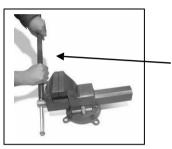
Never Use Cheater Bar in place of the original clamping handle
