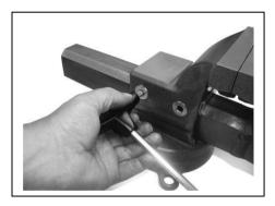
3. Periodically lubricate the V-guides and clamping screw in order to maintain smooth operation and long life.
