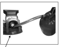
Lubricate Clamping Screws
